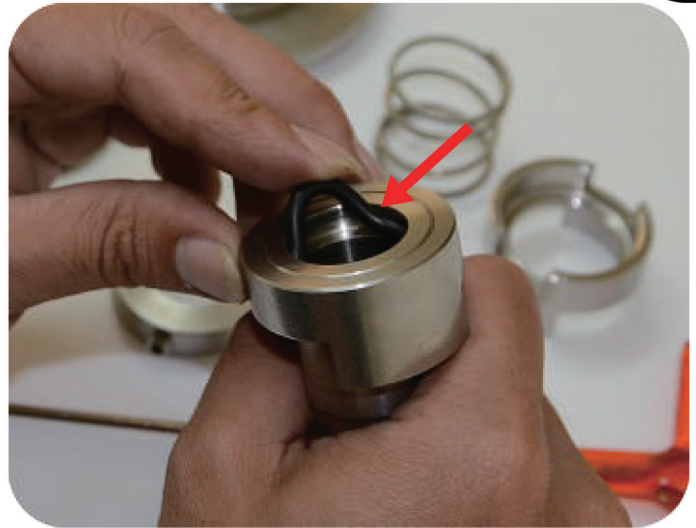
Step1: put O-ring (AS568-114) into the groove of shaft
