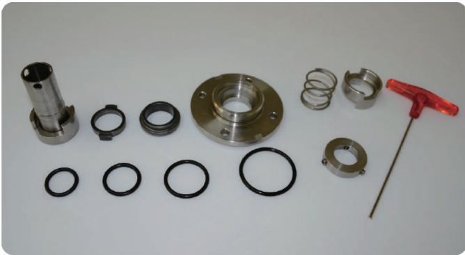
Assemble SB-10,15,20 shaft seal Must be prepared 2.5mm hexagon wrench
