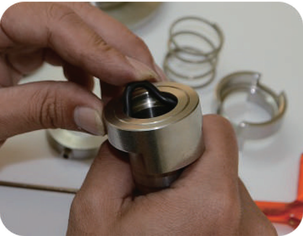
Step9: take out the O- ring ((AS568-114) of spindle *suggest using the tool to assist
