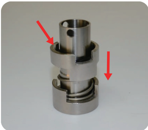
Step4: put the sheath into the shaft
