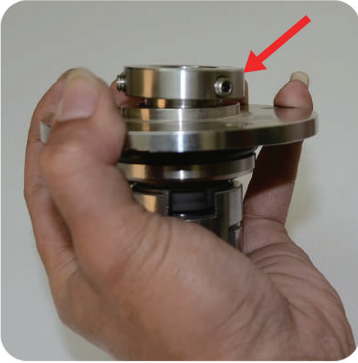
Step10: grasp the set base of shaft seal, put hexagon socket head on it
