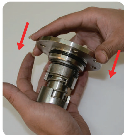
Press the set base of shaft seal and grasp it, avoid the bolt was bounced
