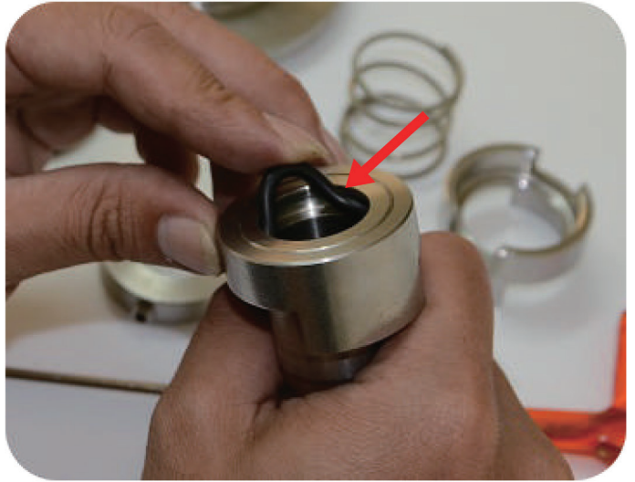
Step1: put O-ring (P22A) into the groove of shaft
