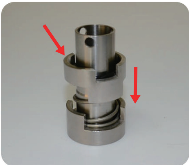
Step4: put the sheath into the shaft
