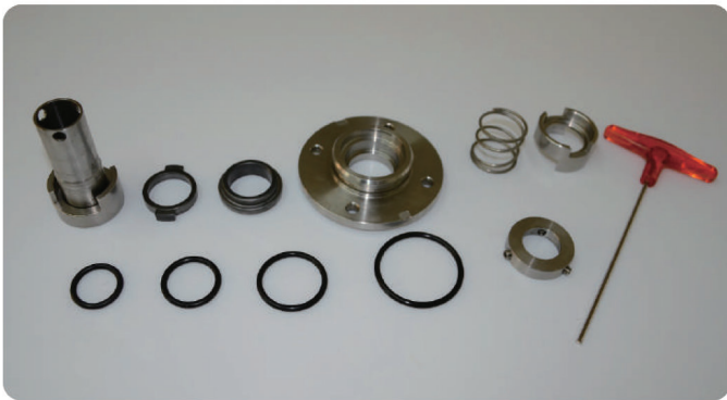
Assemble SB-32,45,64,90 shaft seal Must be prepared 3mm hexagon wrench
