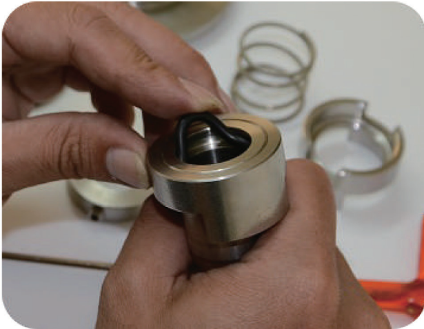
Step9: take out the O- ring (P22A) of spindle *suggest using the tool to assist
