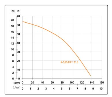
Shaft Speed: 3450 rpm Outlet: 50mm, 2in
